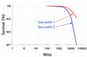
Estimated 'warranty curve' for two user profiles, combines material variability and load variability
