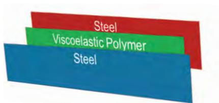
Figure 1: Laminated metals (where two thin sheets of steel or aluminum are bonded together by a thin frequency-dependent damping layer).
